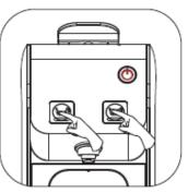
When in "Save Energy Mode", press the two coffee keys together at the same time for 3 seconds and the machine will be ready for setting.
