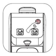
The machine can leave "powersave mode" when power switch is pressed.
