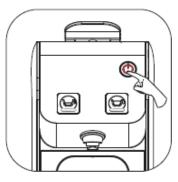
To leave "empty the machine" mode, simply power off or plug off.
