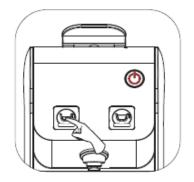
For pre infusion of 1.5 seconds, during "Save Energy Mode", press the small cup key for 3 seconds until you hear the beep sound. you hear the beep sound.
