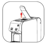
Open the handle and the capsule drops automatically. After brewing, please remove capsule as soon as possible, this will avoid dripping and make dirty infuser.
