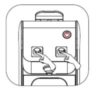
When the machine is ready to be used, press both volume keys together at the same time to empty the machine.
