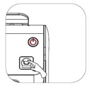
Press lungo key once and the temperature will increase 2 degrees, press twice for 4 degrees and so on. Maximum 8 degrees can be increased.
