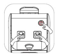
During the Save Energy Mode, press the coffee key and the power key together at the same time for 3 seconds.
