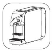
Press Power key and the appliance starts to preheat. Both volume keys blink at 1s/time. Preheating takes about 45 seconds.
