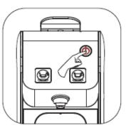
press the power key once to activate the Save Energy Mode manually.
